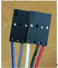
• Next is installing the wires in the 12C port on the Core Device Interface Module. The leftmost pin provides +5V power to the pin, which should map to the VIN pin on the Sensor. The next pin from the left is the I2C data pin, which should map to the SDA pin on the sensor. The next pin from the left is the I2C clock pin, which should map to the SCL pin on the sensor. The rightmost pin is the ground pin, which should map to the GND pin on the sensor.
