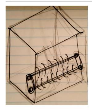
2. In this picture, it shows that the design has shrunk in height. It still has the same amount of space for the storage of the debris.
