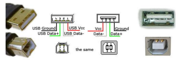
USB is a serial bus. It uses 4 shielded wires: two for power (+5v & GND) and two for differential data signals (labelled as D+ and D- in pinout)
