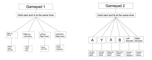
Figure 65.1: Flow chart of controls of Gamepad One (left) and flow chart of controls of Gamepad Two (right).
