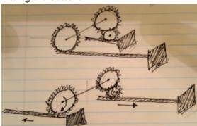
4. In this image, it shows that once a servo motor is put in the middle, the beacon will be able to rotate. Also, if a color sensor is put underneath the servo motor, we can tell which color the rescue beacon is so we can press the correct button.
