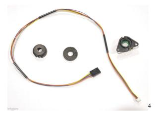
These are the parts of an encoder (shown above). We connect all of these parts to are motor and then it will tell us how fast are motor is going. This can be helpful to tell us information from one format or code to another, to help us understand it better and compare the different motors.
