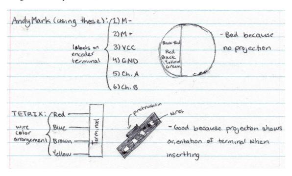
As shown by the sketch, the TETRIX encoder terminal wire colors follow as red-blue-brown-yellow, however this is not the case with AndyMark, where the standard is redblack-red-black-yellow-green. Also, for the AndyMark, the terminal wires have a specific sequence for which wire connects to which input setting. Using this drawing, it is easier to understand to knowing how to connect the TETRIX motor encoders onto the AndyMark DC motors.
