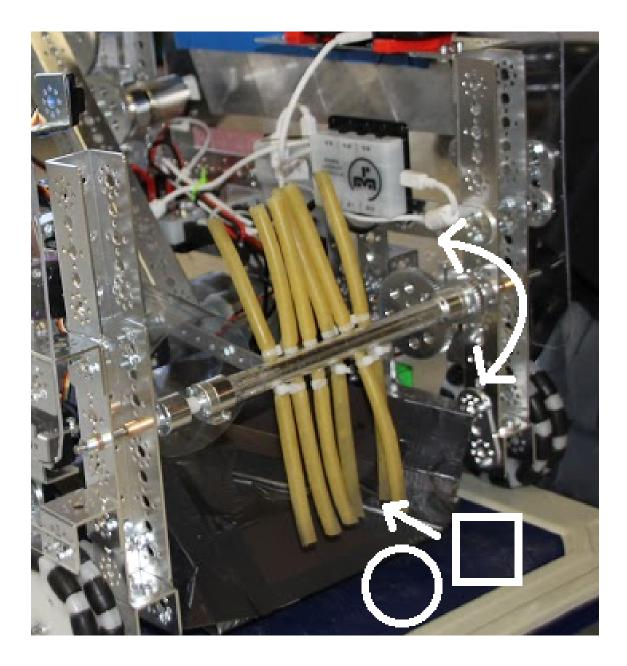
Figure 59.1: The debris collection design implemented on our robot. The debris is to be sweeped in by the sweeper which rotates by a DC motor.
