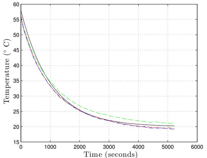
FIG. 3: Results of fitted plot to data. Solid **black** line represents the result from the fitted simulation and dashed lines represent the raw data from the thermocouples. **Red** corresponds to  $x = 0.00$  m, **green** to  $x = 0.075$  m, and **blue** to  $x = 0.15$  m.
