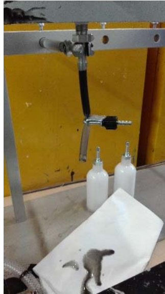
Figure 6: Sealing of the nozzle after filling the mold.
