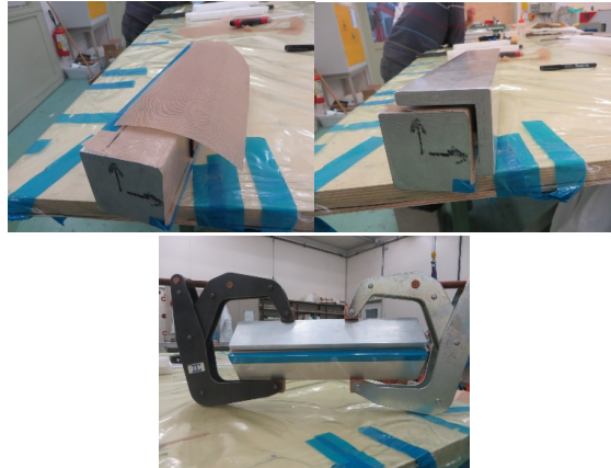
Figure 7: Applying pressure for shape.
