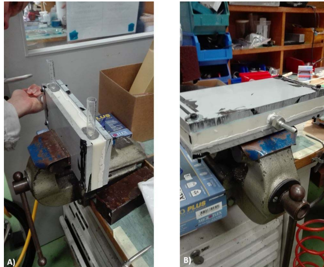
Figure 2: Topmounted plastic tubes (A), The nozzle and the splice sealing silicone added (B).
