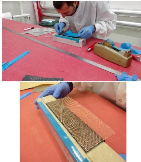
Figure 6: Layers of carbon and copper attached to each other.
