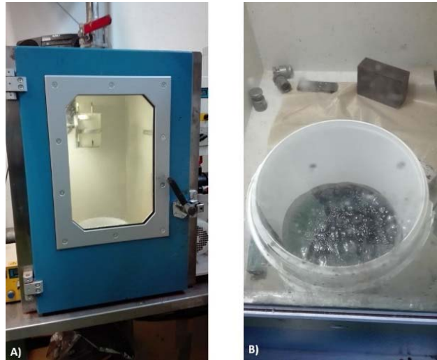
Figure 3: The pressure chamber (A) and the bubbling polymer(B).
