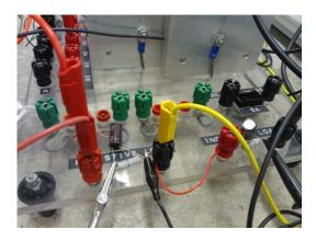
Figure 9: Capacitors across resistors R1 and R2
