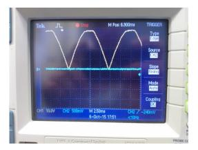
Figure 6: Full wave rectification with no smoothing
