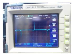
Figure 10: Smoothed output with current spike shown in blue
